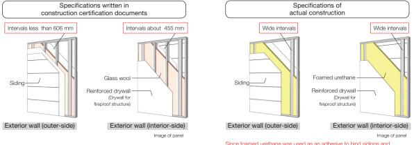
Since foamed urethane was used as an adhesive to bind sidings and reinforced drywall, the intervals between wall backings became wider than the required specifications.
